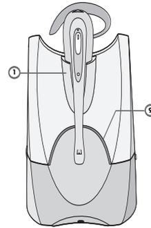
Dock the headset into the charge cradle (1). The amber charge indicator (9) will flash during charge.
