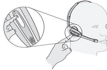
To place a test call press the talk button on the headset.
