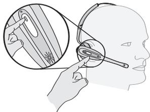
Pressing the talk button (14) on the headset selects headset mode. The talk indicator (2) on the base unit will illuminate steady green and the talk indicator light on the headset will also flash when in headset mode. Both of the indicators are off when in handset mode.
